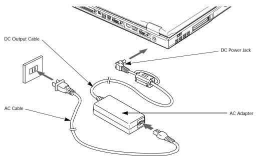
Figure 3-1 Connecting the AC Adapter
